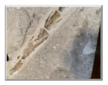
A piece of cut Tyndall stone from Gillis quarry showing the well fossilized internal structure of a Cephlapod. The cavities are also lined with small clear quartz crystals. On the right side of picture shows intricate internal horned coral preserved in the fine grained dark mottled matrix of Dolomite.
